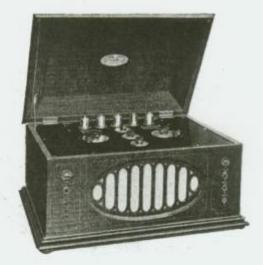
HERE antennae of any and all types may be employed, extraordinary results may be obtained with Radiola VII-B. This Radiola is a five-tube coupled circuit receiver, having two stages of radio-frequency amplification, detector, and two stages of audio-frequency amplification. It employs five UV-199 Radiotrons which operate entirely on dry cells.
